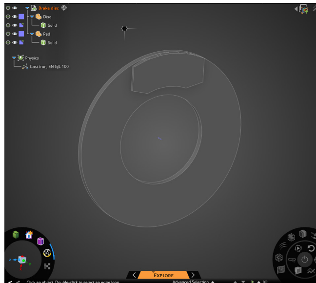
Figure 1: Example CAD file (Disc brake) open in the Ansys Discovery software
